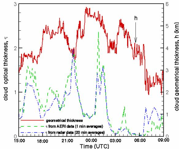
Doppler radar-based estimates of cloud optical thickness typically have errors of about 50-70% which can generally be considered good for a non-optical instrument such as radar.
