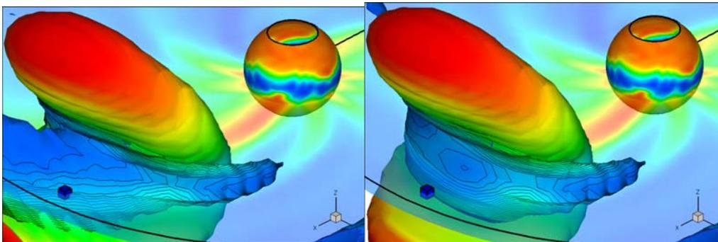
Visualization of an interplanetary disturbance on 15 May 1997 at 00:00 UT for the ICME propagation in steady (left) and evolving (right) solar wind. The solar wind radial velocity is shown on the inner boundary at 30 solar radii, on the injected cloud, and on the translucent equatorial plane using a color scale. The injected cloud (compressed total density) is shown as an iso-surface at  $6 (20) \text{ cm}^{-3}$ . Earth position is shown by the blue box.
