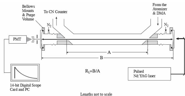
Experimental layout of the Cavity Ring Down System
