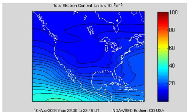
Figure 1. Real-time map of vertical total electron content on August 10<sup>th</sup> 2004 between 2230 and 2245 UT.
