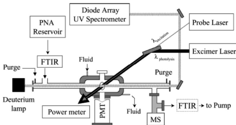
Schematic of the experimental apparatus used to measure the rate coefficients for the reaction of peroxyacetic acid and hydroxyl radical.
