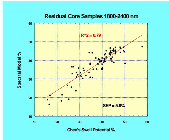
Figure 2. Partial-least-squares regression of spectral reflectance against Chen's swell potential using reflectance spectra from the same core samples used for the engineering tests.
