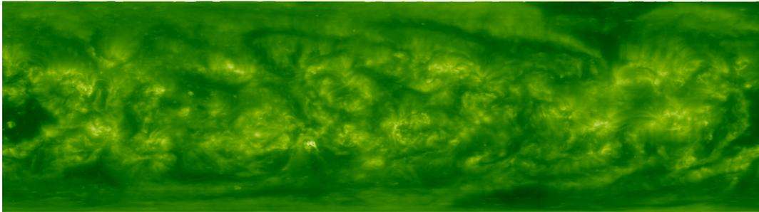
Fig. 2. SOHO/EIT  $\lambda 195\text{\AA}$  synoptic map constructed by the NOAA/SEC generalized synoptic map assembly routine from individual EUV images. Emission maps at this wavelength provide observational reference for coronal hole predictions from the WSA model.
