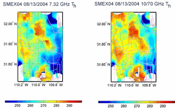
High resolution brightness temperature maps indicating soil moisture content observed over Southern Arizona during SMEX04/NAME experiment.
