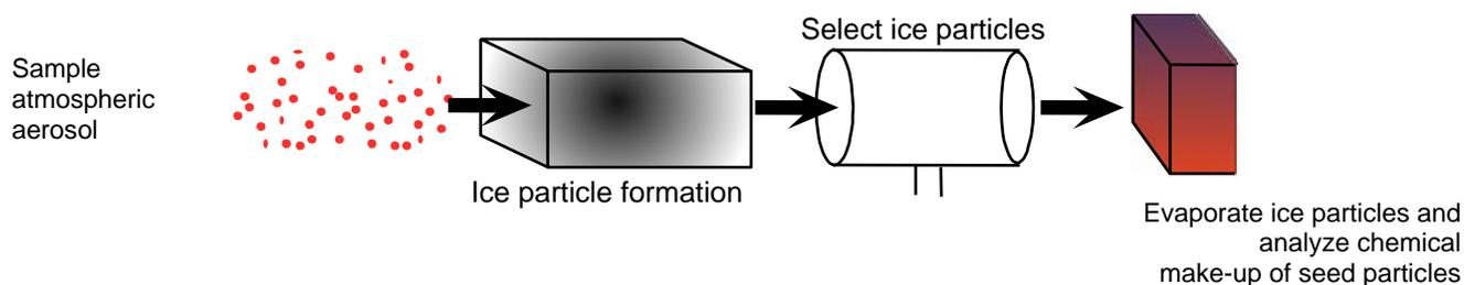
Figure 1 (above). Technique used to determine which atmospheric particles (aerosols) are effective “seeds” for cloud formation
