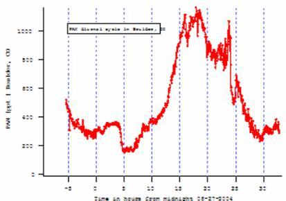
Measurements of PAN over the NOAA Boulder, Colorado laboratory. A chromatogram of PAN of 1000 ppt from outside air at 55 seconds after injection is shown in (a). The peak at 45 seconds is unknown, and the peak at 107 seconds is PPN. One diurnal cycle of PAN during a wet and cool period (high 60, low 50 F) in the summer of 2004 is shown in (b).
