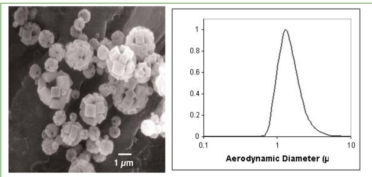
*SEM image and aerodynamic size distribution of microparticles produced by CAN-BD*
