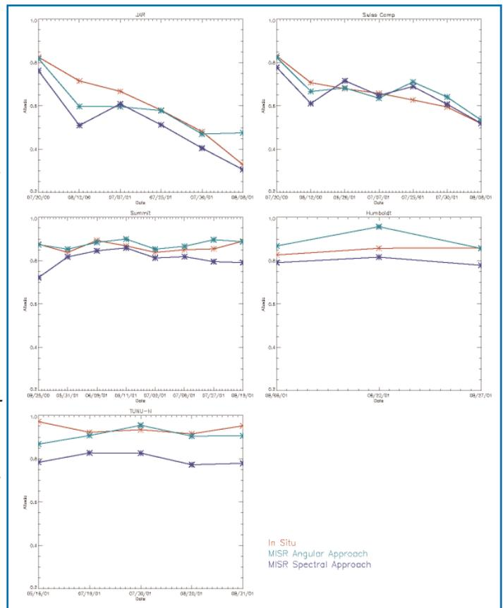
MISR-derived and in situ measured surface albedo at (a) JAR, (b) ETH/CU, (c) Summit, (d) Humboldt and (e) TUNU-N. MISR-derived albedos using both the spectral method (blue) and the angular method (green) are shown.
