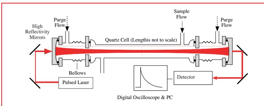
**Cavity Ring-Down Spectroscopy: High-Tech "Photon Ping-Pong" at Work**
