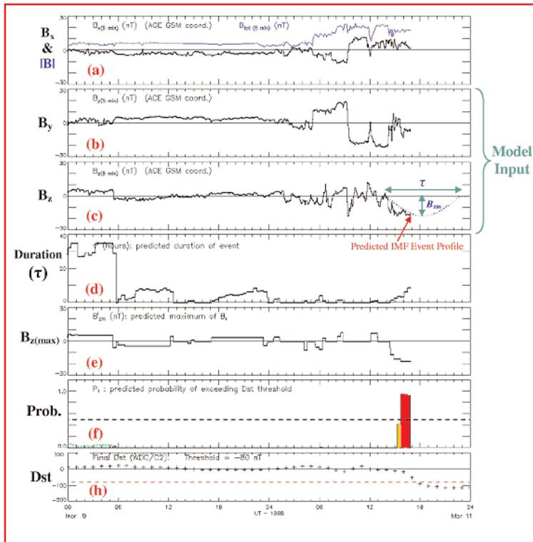
Fig. 2 - Example Chen model prediction: (a-c) IMF field values measured at ACE. (c) predicted IMF event profile (dotted blue sinusoidal curve) (d) predicted IMF event duration (t). (e) predicted IMF event extremum  $B_z$ . (f) Probability of IMF event exceeding Dst threshold. (g) observed Dst. The model successfully predicts, ~1 hour in advance, that Dst threshold will be exceeded.
