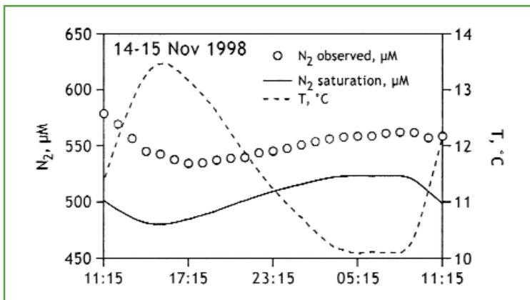
*Illustration of nitrogen supersaturation in a river where denitrification is occurring (South Platte River below Denver).*
