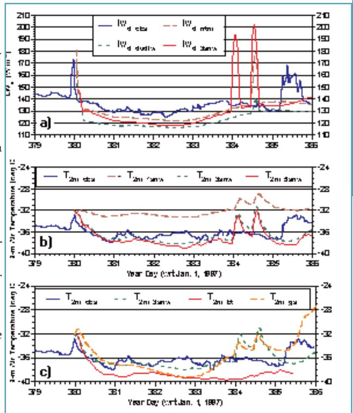
Time series of a) incoming longwave radiation for the radiation tests (DUDLW, RRTM, 3SNW), b) 2-m air temperature for the snow/ice model tests (1SNW, 3SNW, 5SNW), and c) 2-m air temperature for the PBL tests (3SNW, BTPBL, GSPBL) for January 14-20, 1998. The heavy solid curves are observed values in all panels
