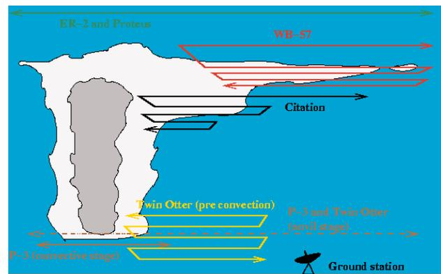
*Schematic showing how a tropical cirrus cloud will be sampled with a suite of six aircraft and ground measurements planned for the CRYSTAL-FACE mission.*
