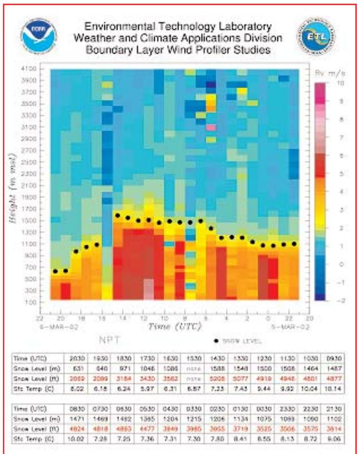
*Example of the snow level web display produced from profiler data recorded at Newport, Oregon on 5 March, 2002. The colored rectangles indicate values of Doppler vertical velocity ( $R_v$ ; positive downward). The snow level algorithm output is indicated by the black dots.*
