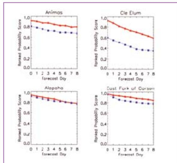
*This figure summarizes the skill of our experimental streamflow forecasting system (red triangles, solid line) versus the traditional ESP approach (blue squares, dotted line) in terms of the ranked probability skill score. Results are shown for four river basins nationwide: the Animas River in southwestern Colorado, the Cle Elum in central Washington, Alapaha River in southern Georgia, and the east fork of the Carson on the California/Nevada line.*
