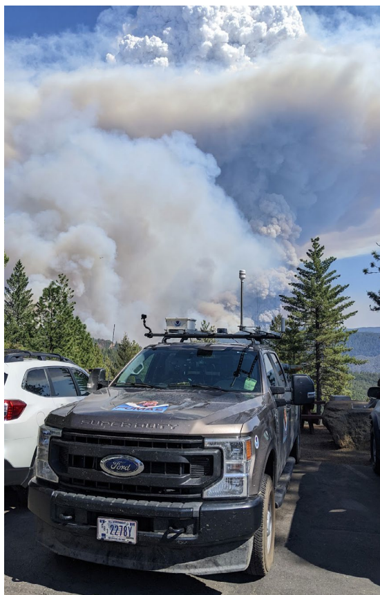
While the Twin Otter flew above, researchers drove trucks around the perimeter of the Mosquito Fire to measure wind speed and air temperature. Photo: Richard Marchbanks/CIRES and CSL
