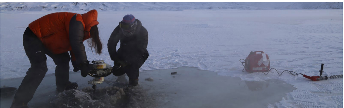
Researchers use an auger to test for water flowing beneath river ice during winter in southwest Greenland. Photo: Lincoln Pitcher/CIRES
