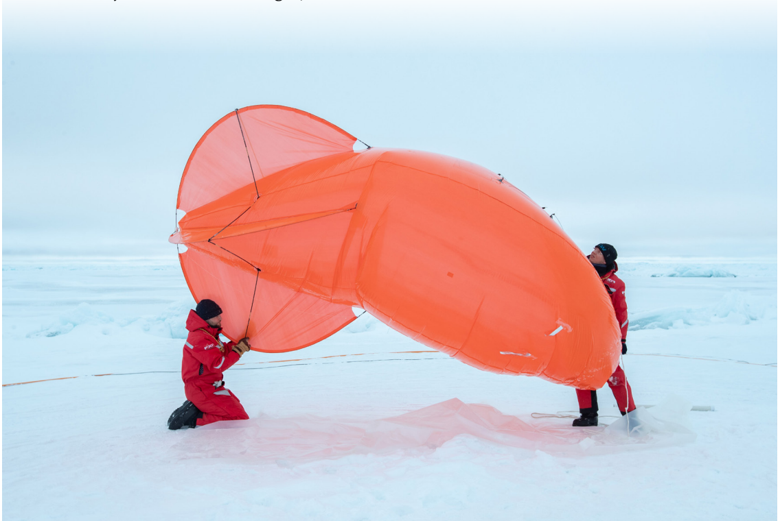
Atmospheric scientists Alex Schulz and Sandro Dahlke deflate 'Miss Piggy', a weather balloon used to deploy instruments that help the scientists understand atmospheric properties like temperature and turbulence. Photo: Lianna Nixon/CIRES and CU Boulder
