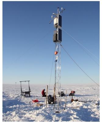
The AMIGOS-III A tower was installed on the Thwaites Ice Shelf. The tower stands roughly seven meters (23 feet) above the snow surface to allow it to operate through two-to-three years of snow accumulation. Photo: Ted Scambos/CIRES
