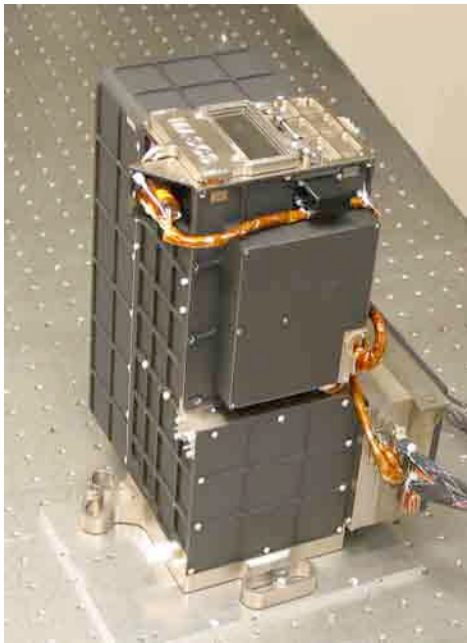
Figure: The MASCS detector package that is being prepared for MESSENGER by LASP researchers.
