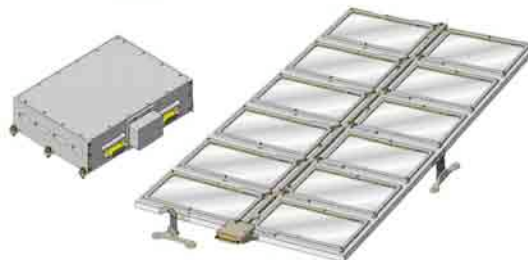
Figure: The mechanical configuration of the SDC/CDE instruments. SDC will map the dust distribution in our Solar System from 1 to >50 AU, while CDE will monitor the dust influx into the Earth's atmosphere. The Cosmic Dust Experiment (CDE) is part of the Aeronomy of Ice in the Mesosphere (AIM) Mission.
