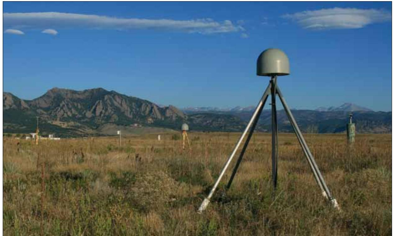
Early-morning lenticular and stratus clouds form over the foothills in Boulder, Colorado. High-rate Global Positioning System (GPS) receivers, such as the one in the foreground, can help scientists detect the amount of moisture in the soil, which improves weather and flood forecasting. (Courtesy N. Vizcarra)
