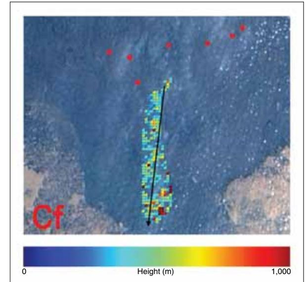
This image from the Multi-Angle Imaging Spectroradiometer (MISR) instrument, on board the NASA Terra satellite, helped researchers trace the source of a heavy smoke plume over Cairo, Egypt. The colored spots indicate plume height measurements, with abundant bright blue-green spots showing that the smoke mostly resided in the lower 500 meters (1,600 feet) of the atmosphere. The arrow pointing south shows the direction that the plumes were drifting. (Courtesy H. Marey et al.)
