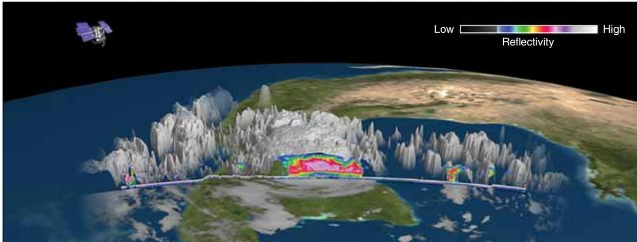
The NASA CloudSat satellite captured a slice of Hurricane Karl's clouds at 8:01 a.m. GMT (4:01 a.m. EDT) on September 17, 2010. CloudSat shows that the clouds are over eight miles high. The blue areas along the top of the clouds indicate cloud ice. The highest clouds in Karl at the time of the image were as cold as -40 to -60 degrees Celsius (-40 to -76 degrees Fahrenheit). (Courtesy NASA/JPL/Colorado State University/NRL)
