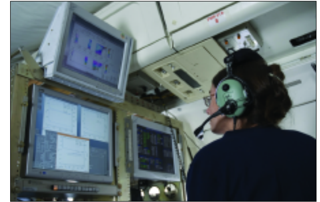
Susan Kool monitors data from the Lidar Atmospheric Sensing Experiment (LASE) instrument on board a NASA DC-8 aircraft flying through a Saharan dust storm over the Atlantic. Researchers hope to use these data to track interactions between the dust and tropical storms and to better understand Atlantic hurricane development. (Courtesy NAMMA team)
