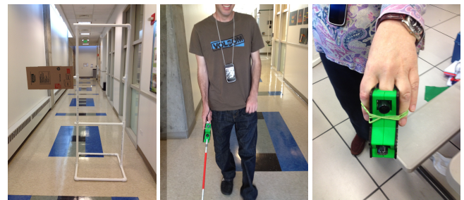
Figure 7: From left: A picture of the obstacle rig (set at medium height), a user with the ioCane and phone around the neck, and a user trying the ioCane as a handheld device.
