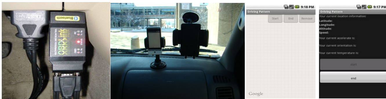
Figure 6: OBD and personal mobile devices deployed in vehicles for real-time monitoring.
