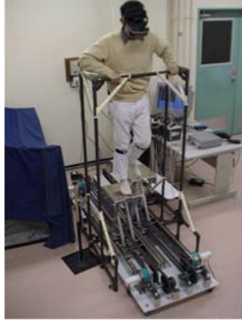
Figure 7. GaitMaster keeps a user’s legs on the movable pedals [28].
