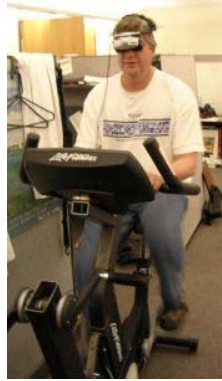
Figure 2: Recorded surround video and terrain features are played back on synchronized HMD and exercise bike.
