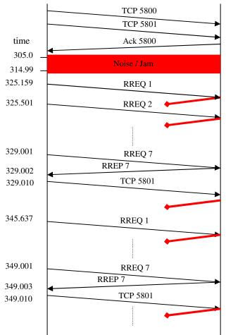
Figure 3: Simulated jamming attack on AODV/TCP
