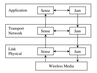
Figure 1: The sensing and jamming layered model
