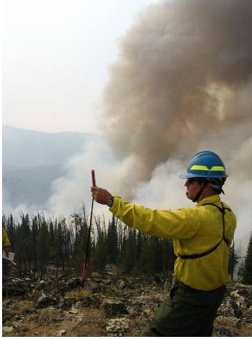
Figure 1: A fire fighter takes wind measurements using a belt-weather kit.
