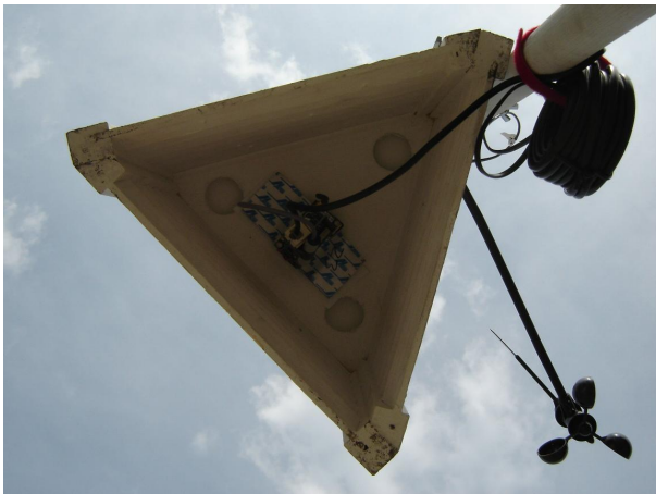
(b) Nodes were attached to the ceiling with industrial velcro. All sensors faced down towards the open bottom.
