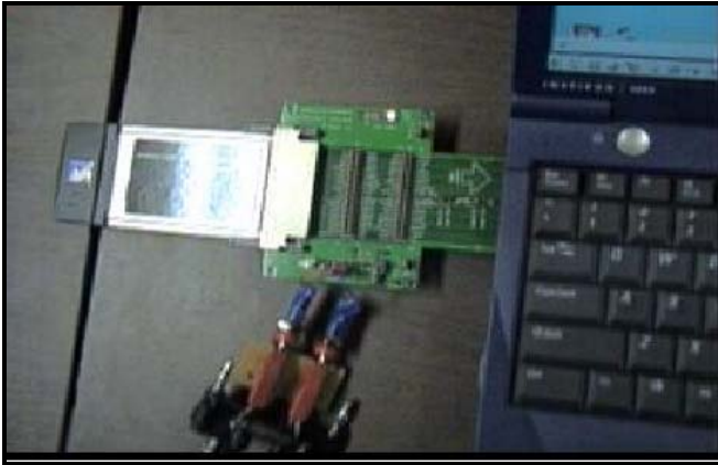
Figure 10: Picture of the setup to measure power consumption.
