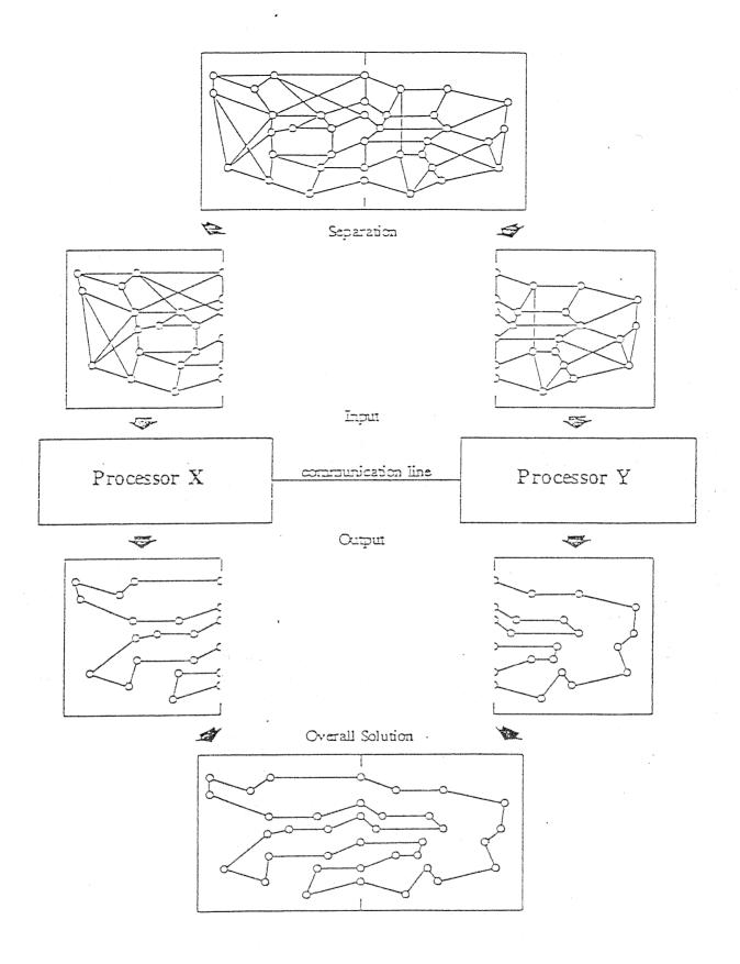
Figure 1. Two processors, solving a graph problem. The cut size is 6.
