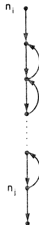
FIGURE 16. Pathological situation in which the execution time for the availability algorithm is unusually long. Here d = |N| - 3 , \tau = (|N| - 1)^2 assuming \alpha \in \text{gen}(n_i) and \alpha \in \text{kill}(n_j) and is not in any other gen or kill sets.
