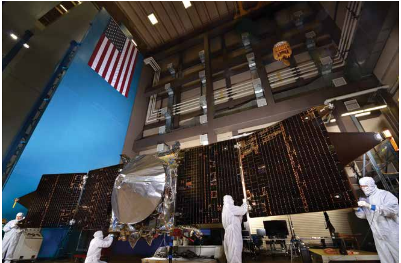
Before it heads to Mars, NASA's MAVEN spacecraft tests its solar arrays during environmental testing at Lockheed Martin's facility near Denver, Colo. MAVEN will perform the first dedicated mission to survey the upper atmosphere of Mars.
