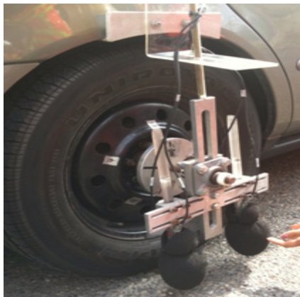
OBSI Apparatus (portable, can be used with any vehicle)
