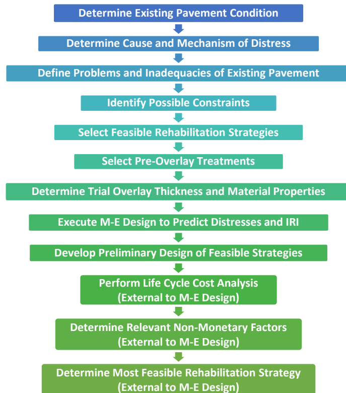
Figure 8.1 Rehabilitation Alternative Selection Process
