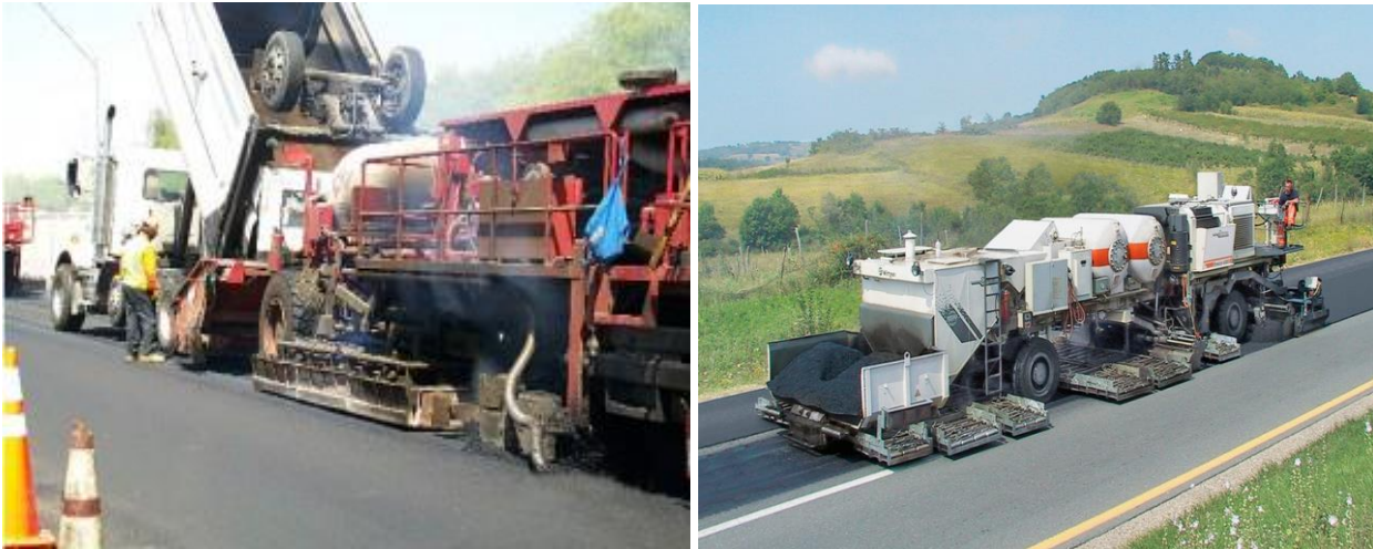
Figure 8.18 Photos of Heating and Remixing Equipment
