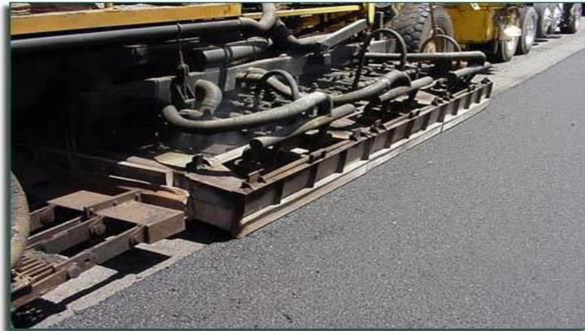
Figure 8.15 Photo of Heater Section of the Equipment Train
