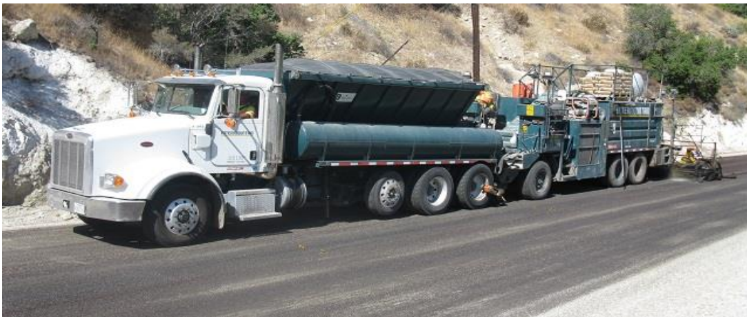
Figure 8.29 Photo Showing Micro-Surfacing Equipment
