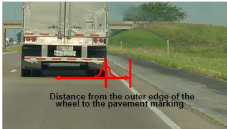
Figure 3.15 Schematic of Mean Wheel Location
