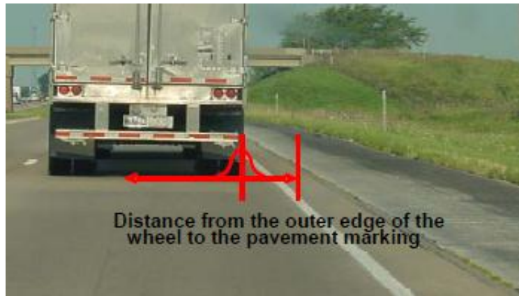
Figure 3.15 Schematic of Mean Wheel Location
