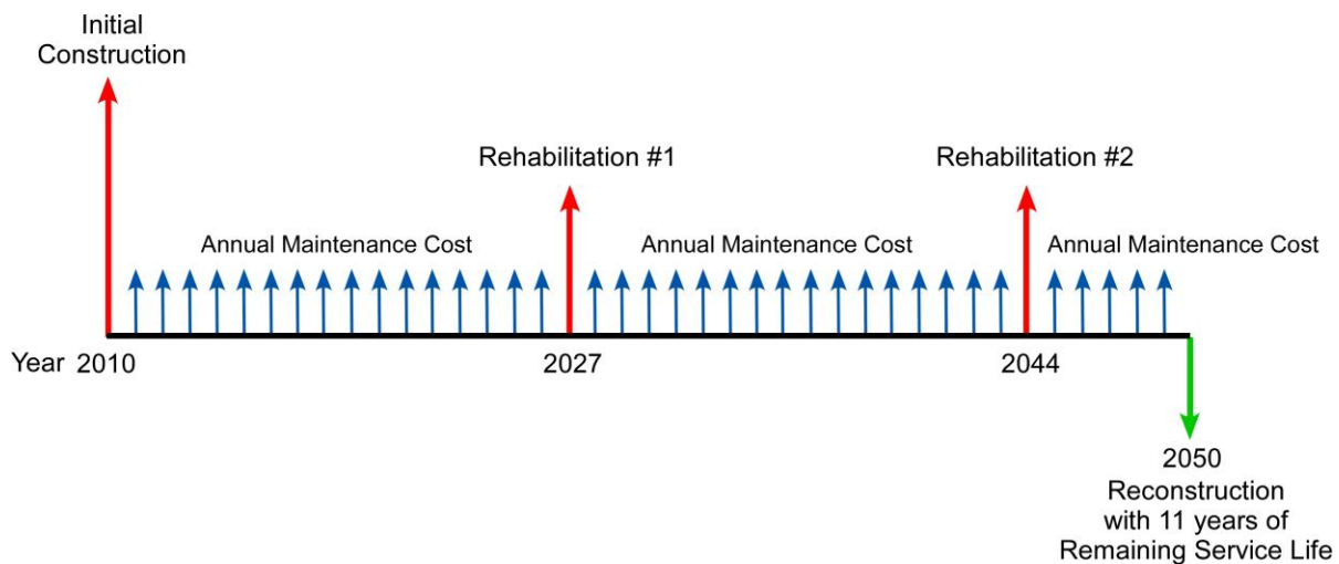
Figure 13.2 Unmodified HMA Cash Flow Diagram
