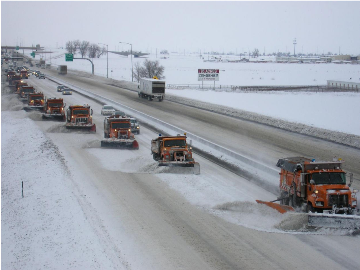
CDOT crews plow I-25 in tandem to pull snow away from areas such as walls and medians where drainage is poor. Snow and ice removal is a customer service CDOT offers that directly affects the traveling public.
