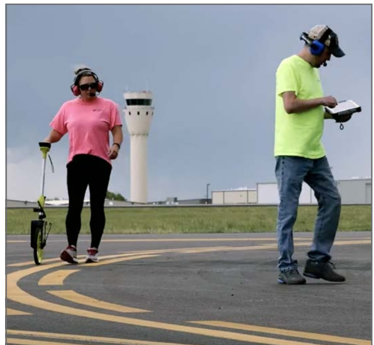
The Division's Aviation Planners Kaitlyn Westendorf (left) and Scott Storie (right) perform a Pavement Condition Index (PCI) inspection at Centennial Airport (APA).
