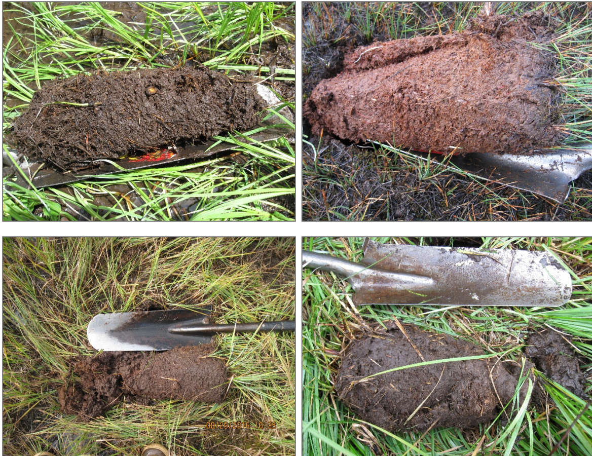
Figure 3. Examples of organic soil. Note the presence of roots and fibric organic material throughout the soil core. Color may be dark brown to reddish brown depending on source material. Soil holds together.
