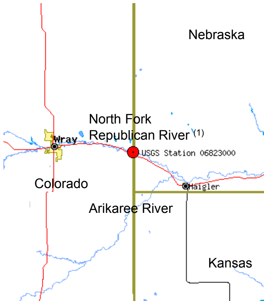
(1) Haigler Canal diverts flow upstream of station in Colorado; return flows enter Arikaree River in Nebraska
