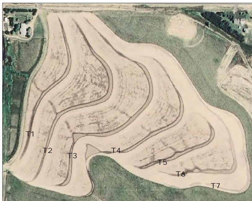
Figure 23. FSA digital photograph of a terraced field used to illustrate the use of a field-grade GPS system to characterize field conditions and terrace storage.
