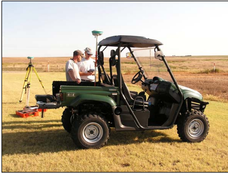
Figure 3. Picture of the all terrain vehicle and survey-grade GPS system used to survey terrace conditions.
