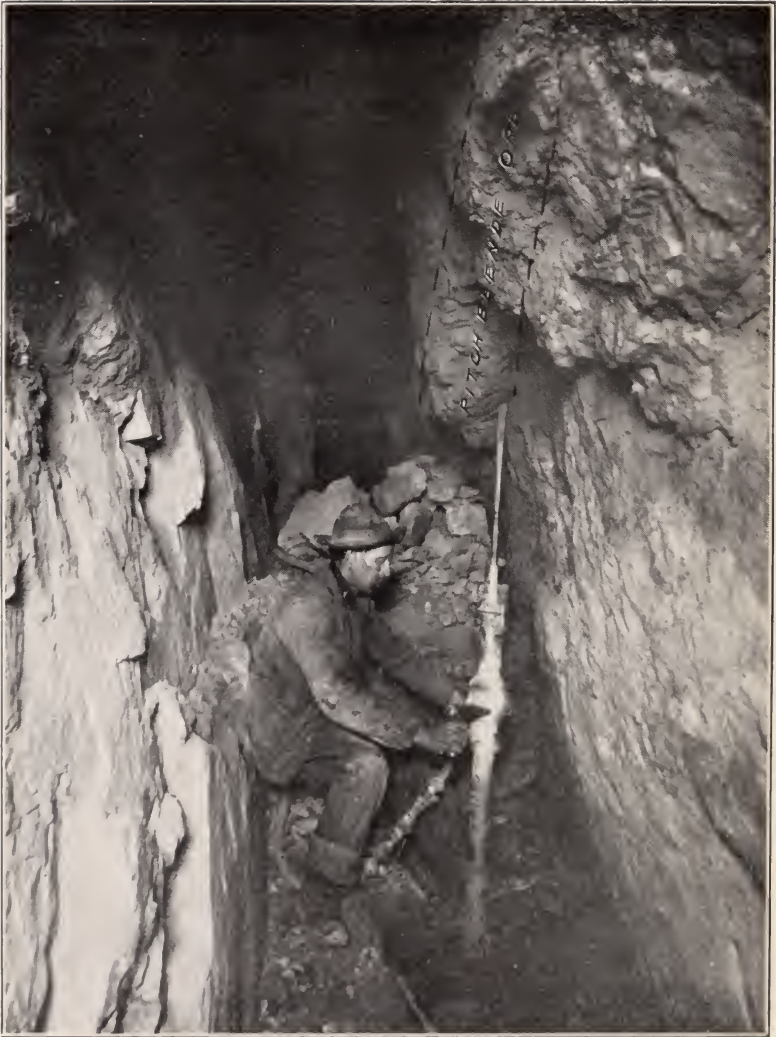
Showing Vein of Pitchblende Ore in a Gilpin County Mine, 800 Feet Underground. The Miner is Operating a Machine Drill.
