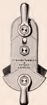
STEPHEN HUMBLE'S DETACHING HOOK WITH COPPER RIVET HOLD- ING SAME IN POSITION FOR HOISTING.
