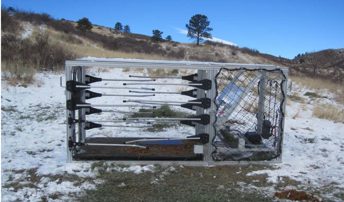
Figure 3. Device frame. The sides of the device comprise one-way gates that prevent entry to the device yet allow animals to easily exit once inside. Animals will be required to enter the device through a 14" x 32" opening in the front, which is adjustable. The rear portion of the device is a bait compartment fabricated from aluminum. A door on the rear of the bait compartment will allow biologists to easily add bait in the field and access controls.
