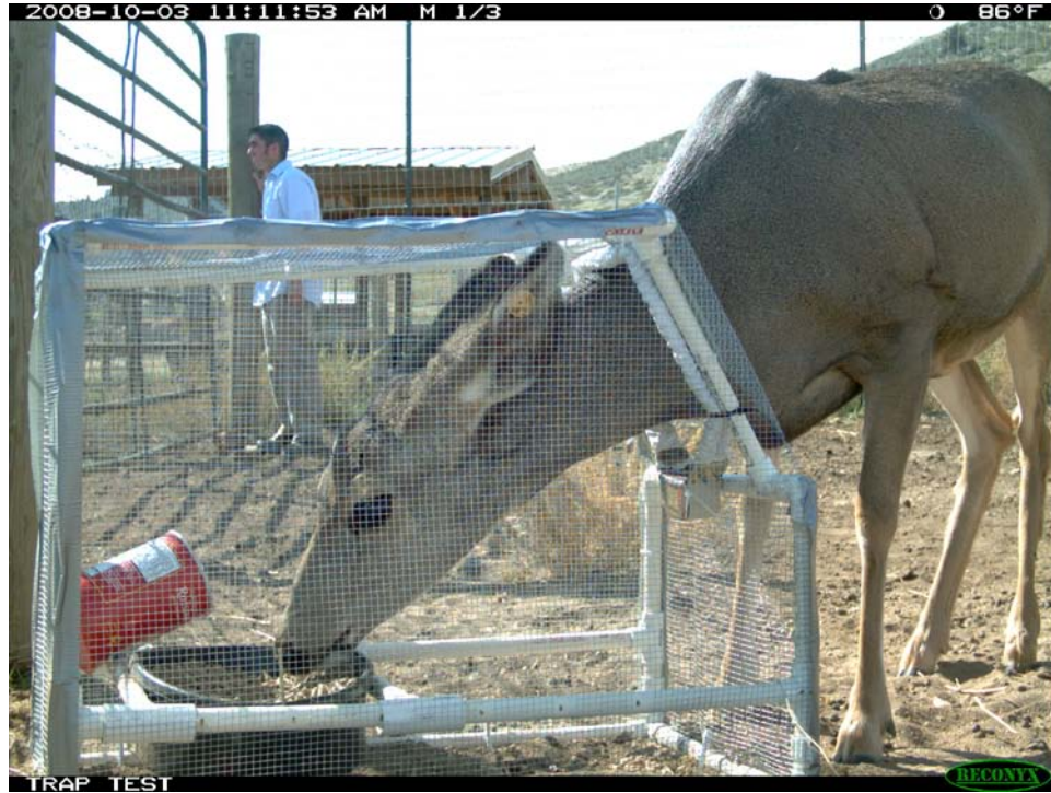
Figure 1. Prototype evaluation of collar and bait placement, and validation that a deer would extend its head and neck through an expanded collar to access the bait.
