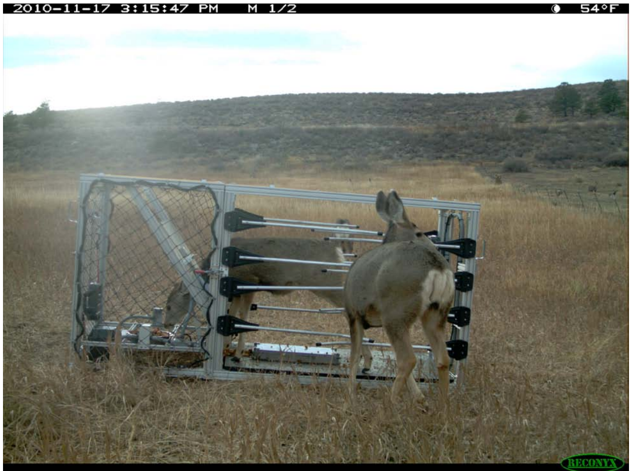
Figure 1. Automated collaring device for mule deer, comprising an aluminum cage and a bait compartment. Deer become collared by entering the cage and extending their head through an expanded radio collar when accessing bait.
