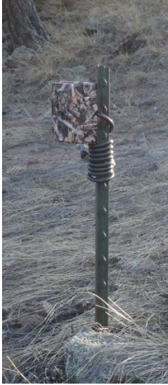
Figure 2: For randomly selected sites with no available trees, camera units are installed on a T-post with a bracket custom made for the unit.
