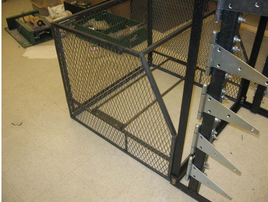
Figure 4. The bait compartment. Deer will be required to extend their head and neck through an outstretched expandable radio collar in order to reach the bait.
