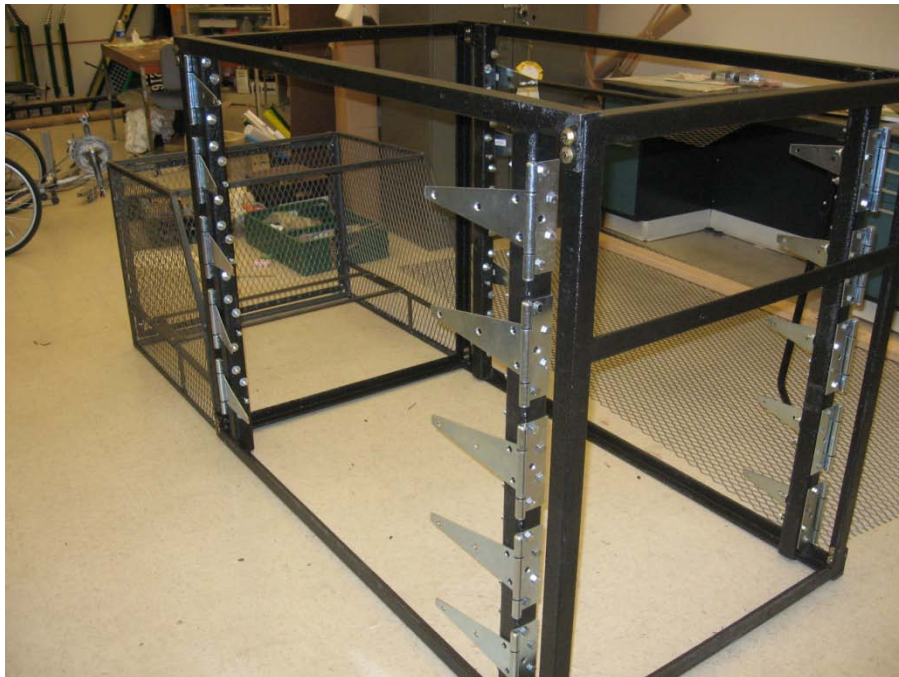
Figure 3. Device frame. The sides of the device will comprise one-way gates that prevent entry to the device yet allow animal to easily exit once inside. Animals will be required to enter the device through a 14" x 32" opening in the front. The rear portion of the device is a bait compartment fabricated from steel. A door on the rear of the bait compartment will allow biologists to easily add bait in the field.
