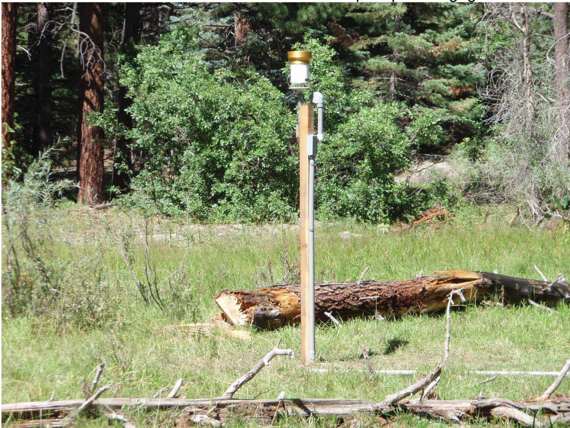
Precipitation gage installed at the East Fork of the San Juan stream gage. Rain gage is located in an open meadow above the stream gage.
