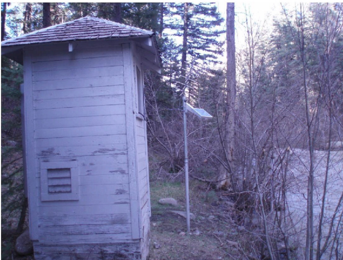
Refurbished USGS Gage on the East Fork of the San Juan River to monitor the landslide
