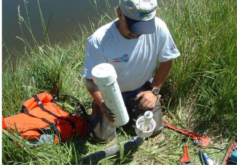
Muffler Installation at the Williams Fork Gage Station
