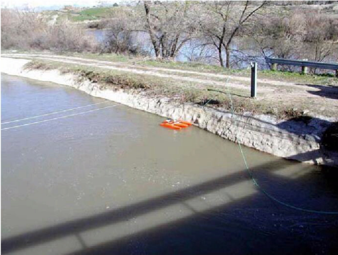
ADCP Stream Pro at Redlands Power Canal near Grand Junction
