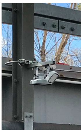
The OTT RLS and OTT SVR 100 fixed to a bridge over flowing water.
