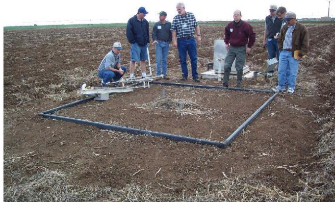
Similar Weighing Lysimeter as installed at Bushland, Texas
