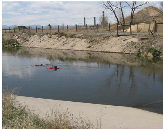
ADCP deployed at BURCANCO June 6, 2008
