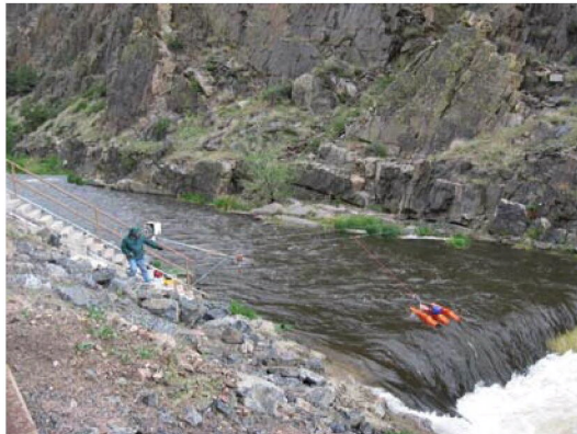
ADCP deployed at Big Thompson River at Canyon Mouth
