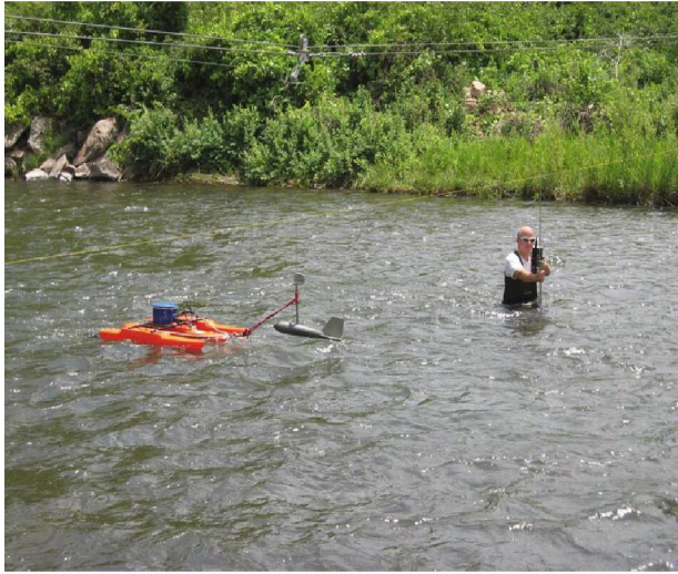
ADCP measurement alongside a Current Meter measurement made by Patrick Tyler at South Platte River at Waterton, CO (PLAWATCO)
