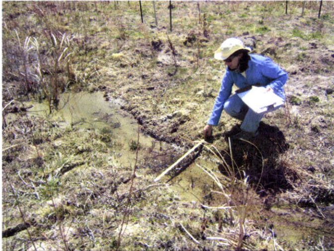
Suzanne Sellars obtaining a low flow measurement at Woodmen Hills.
