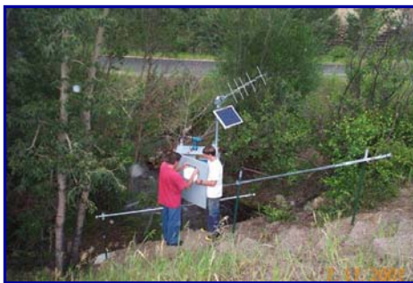
Fall River near Idaho Springs — A new installation funded by the CWCB tracks minimum stream flows.
