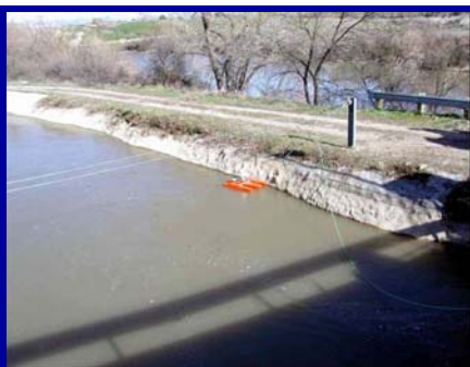
ADCP Stream Pro at Redlands Power Canal near Grand Junction
