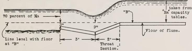
**First**—Select from Table of flume capacities, the proper depth of water or head "Ha" that corresponds with the maximum capacity of the ditch, so that "Ha" will ordinarily not exceed one-half of the width of throat "W" which may be adopted.
