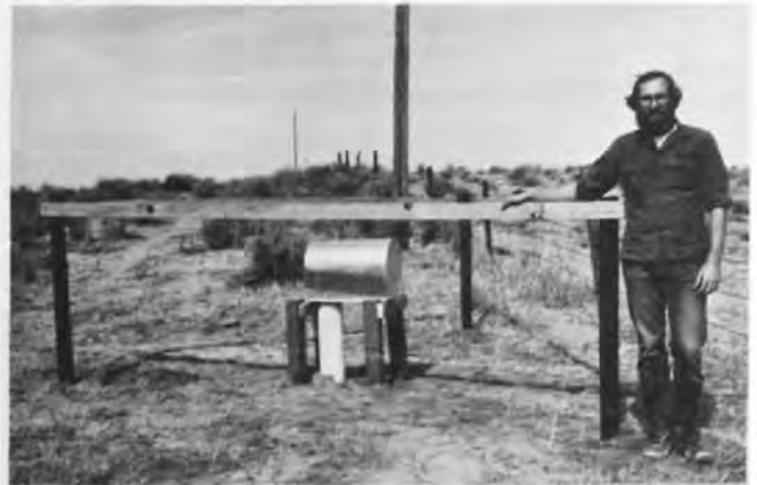
Photo 4. Recorder well with recorder installed in metal house and protected by a fence.
