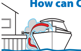
Blocked exhaust outlets
