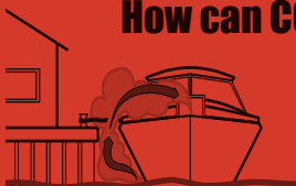
Blocked exhaust outlets
