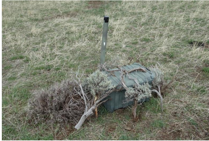
Figure 9. The datalogger setup in the waterproof box with the lid closed and camouflaged with sagebrush in the Axial Basin area of Moffat County, Colorado, 2018.
