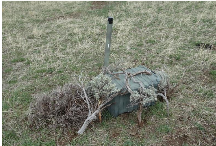
Figure 4. The datalogger setup in the waterproof box with the lid closed and camouflaged with sage on SG4/Collom 2 lek in northwestern Colorado.
